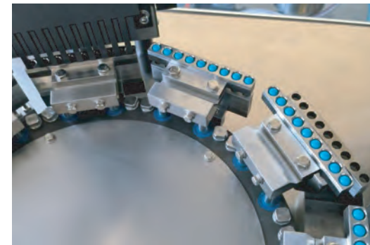
Powder Filling Station
