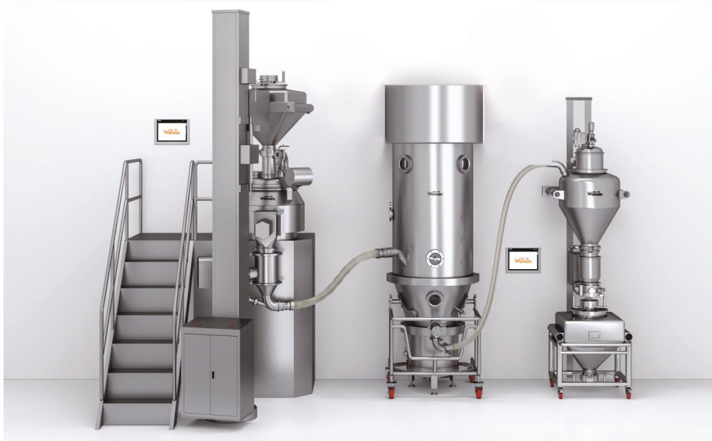
10-200kg Containment granulation line
