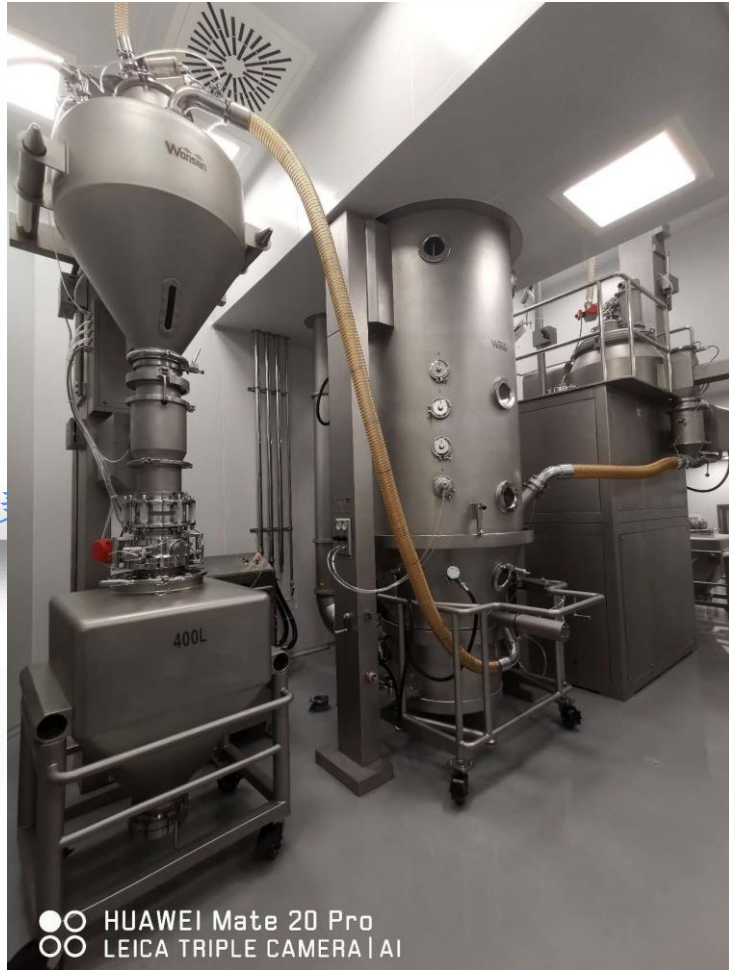
Morocco granulation line OEB4 (120kg)
